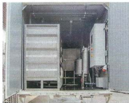
Blick in den mobilen Wasser-Recycling-Container
